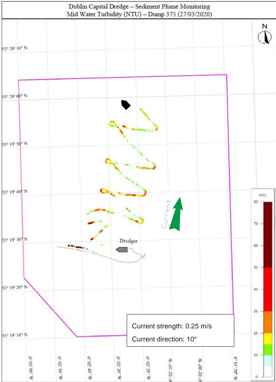
Figure 8.31: Dump 375 Survey track with mid water turbidity [NTU]
