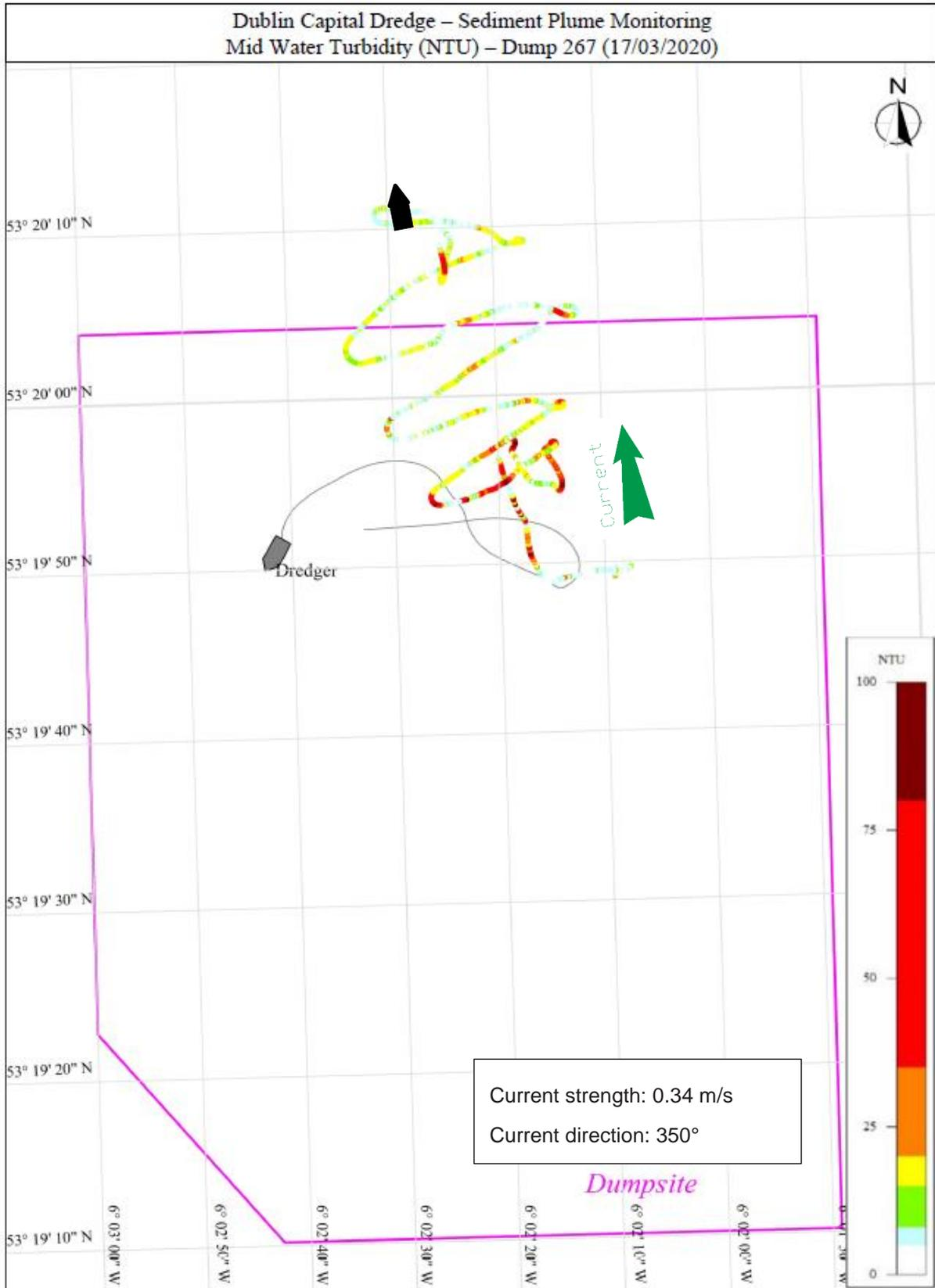
Figure 8.6: Dump 267 Survey track with mid water turbidity [NTU]
