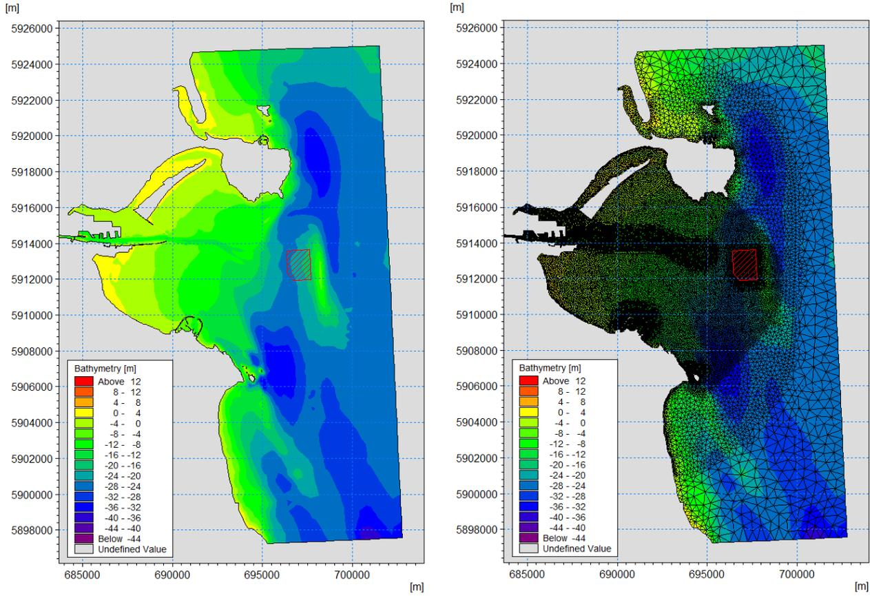
Figure 4.1: Extent and bathymetry (left) and mesh structure (right) of the Dublin Bay model. Location of the licenced dump site shown by red hatch area.
