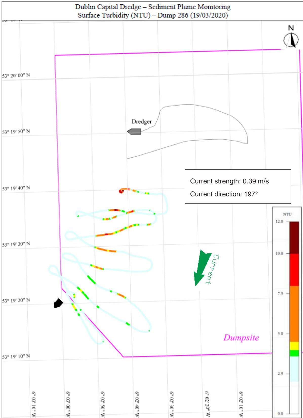
Figure 8.19: Dump 286 Survey track with surface turbidity [NTU]
