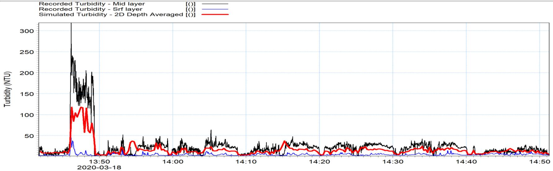
**Figure 8.40: Comparison of recorded and simulated turbidity measurements across the dump site during Event 283**
