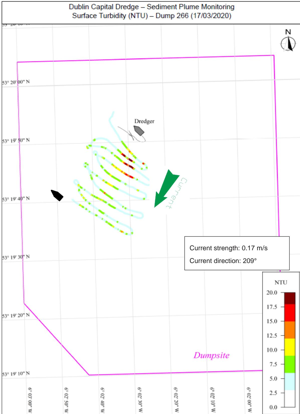
Figure 8.3: Dump 266 Survey track with surface turbidity [NTU]
