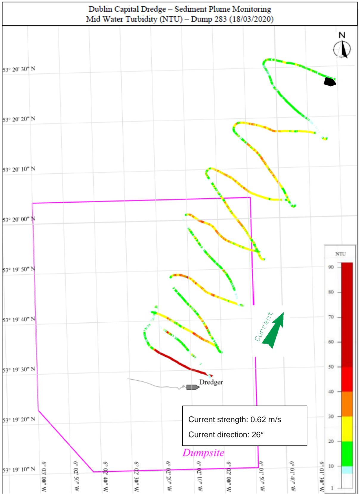
Figure 8.15: Dump 283 Survey track with mid water turbidity [NTU]
