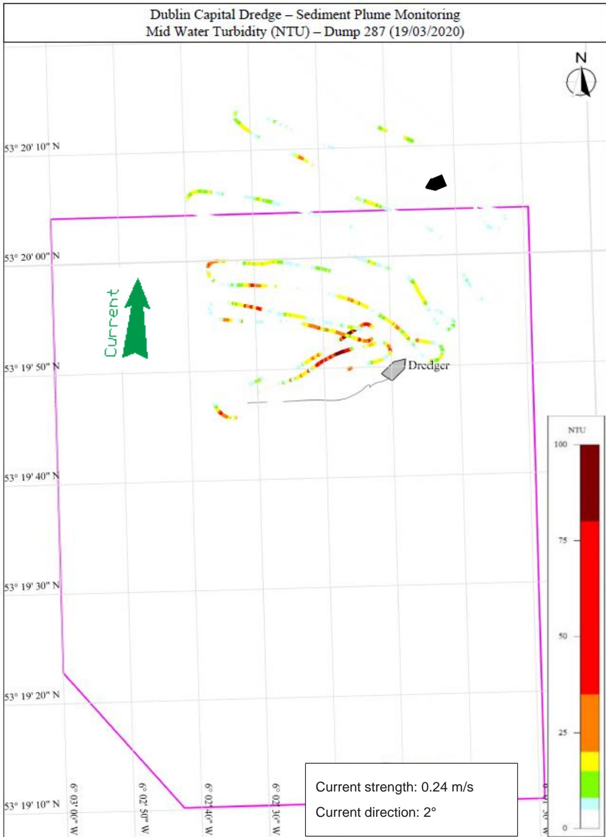
Figure 8.22: Dump 287 Survey track with mid water turbidity [NTU]
