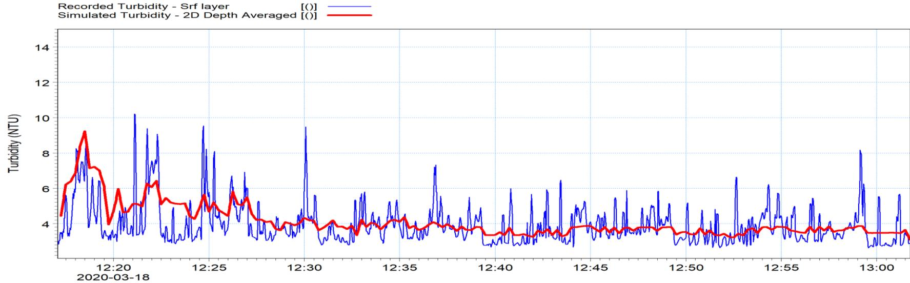
**Figure 8.39: Comparison of recorded and simulated turbidity measurements across the dump site during Event 282**
