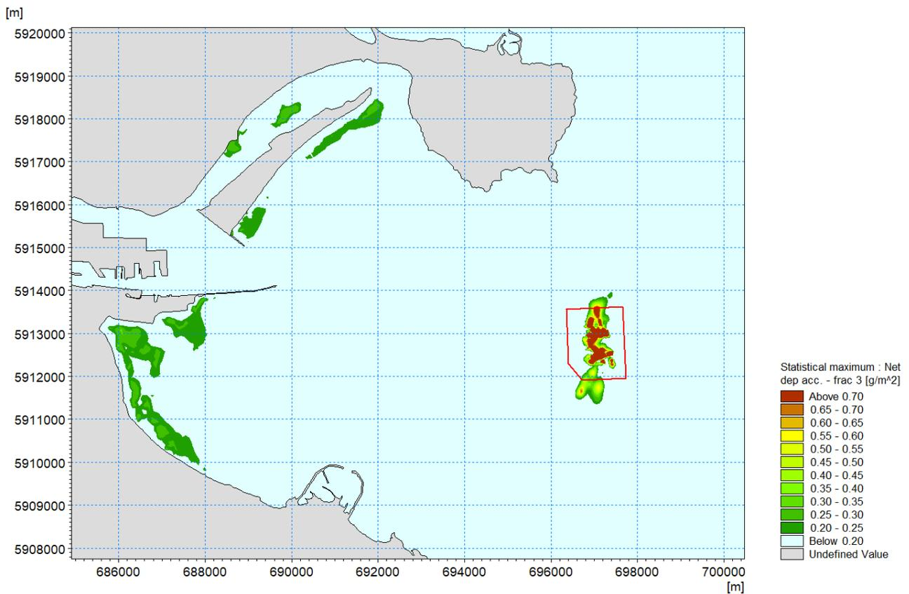
**Figure 4-7 Total deposition of silt material following the dumping at sea activities associated with the Dublin Port 2022 - 2029, Maintenance Dredging Programme (S0004-03)**
