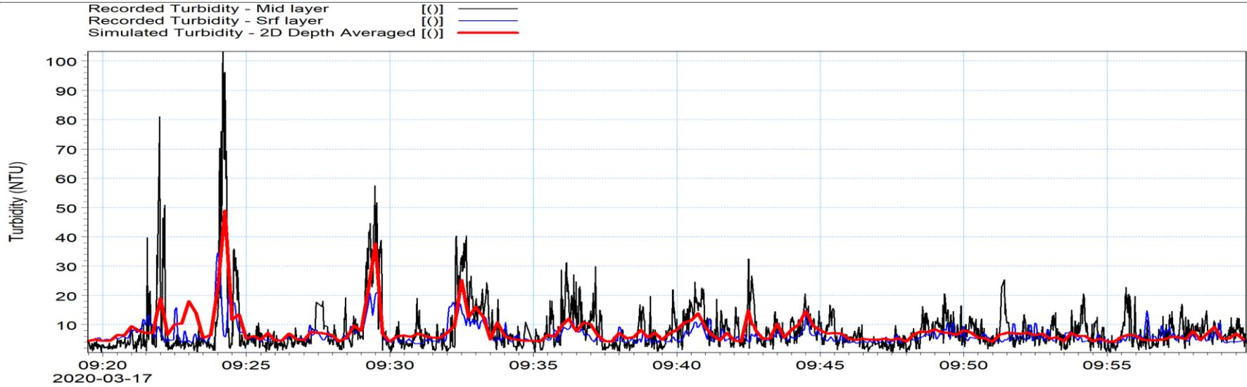
**Figure 8.34: Comparison of recorded and simulated turbidity measurements across the dump site during Event 266**
