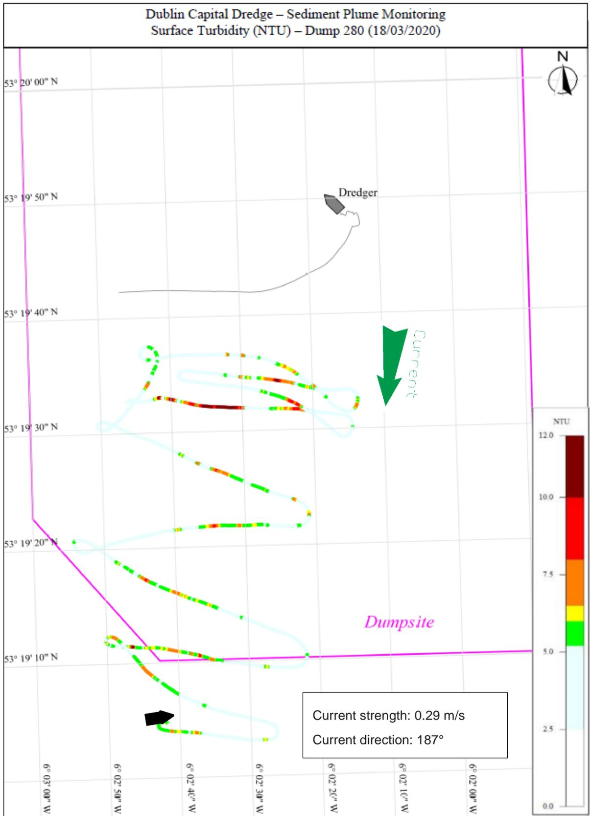
Figure 8.9: Dump 280 Survey track with surface turbidity [NTU]
