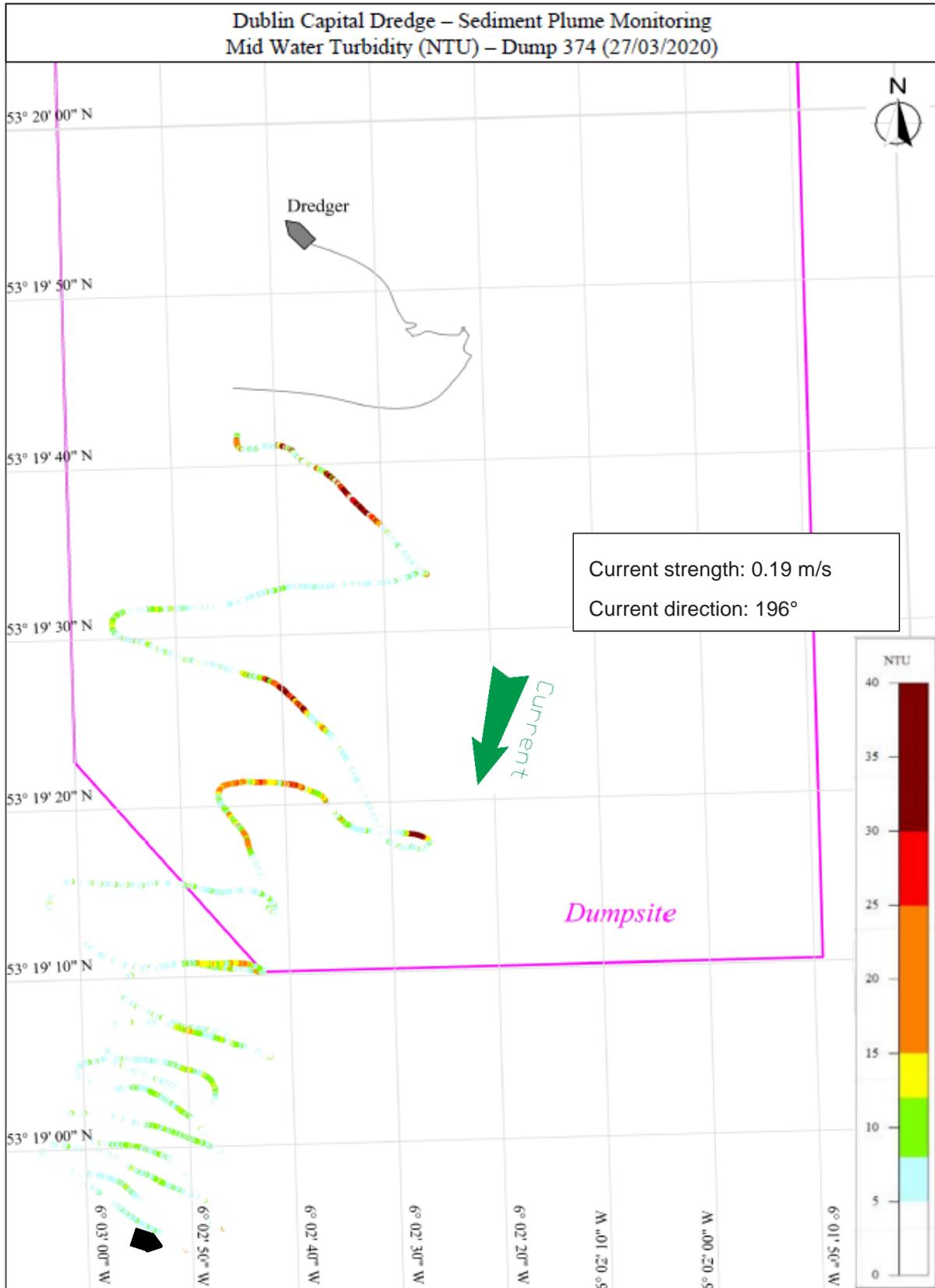
Figure 8.29: Dump 374 Survey track with mid water turbidity [NTU]
