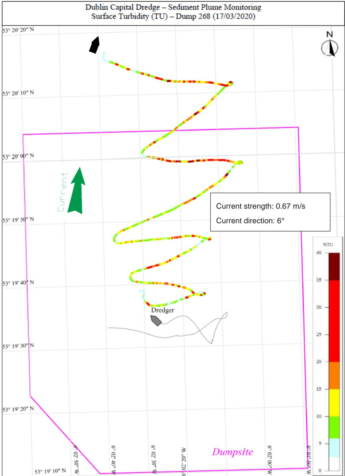
Figure 8.7: Dump 268 Survey track with surface turbidity [NTU]
