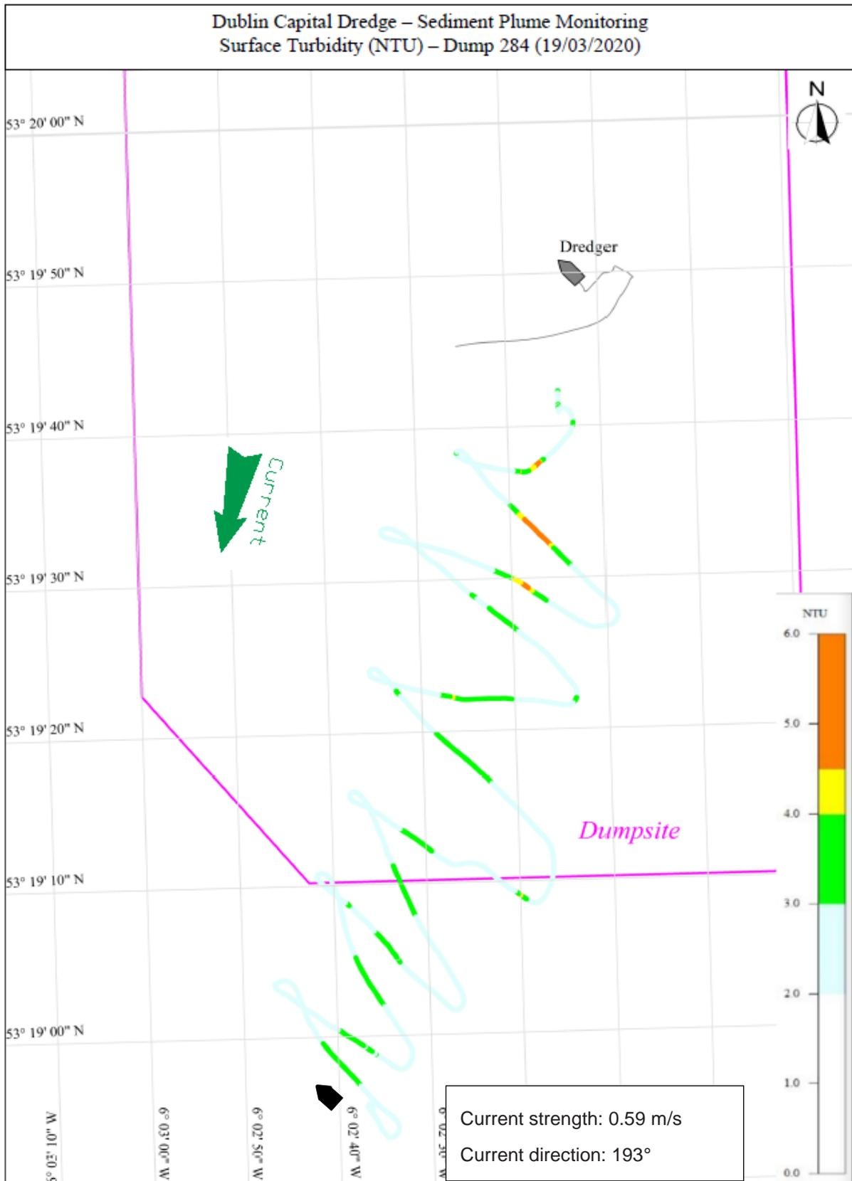
**Figure 8.16: Dump 284 Survey track with surface turbidity [NTU]**
