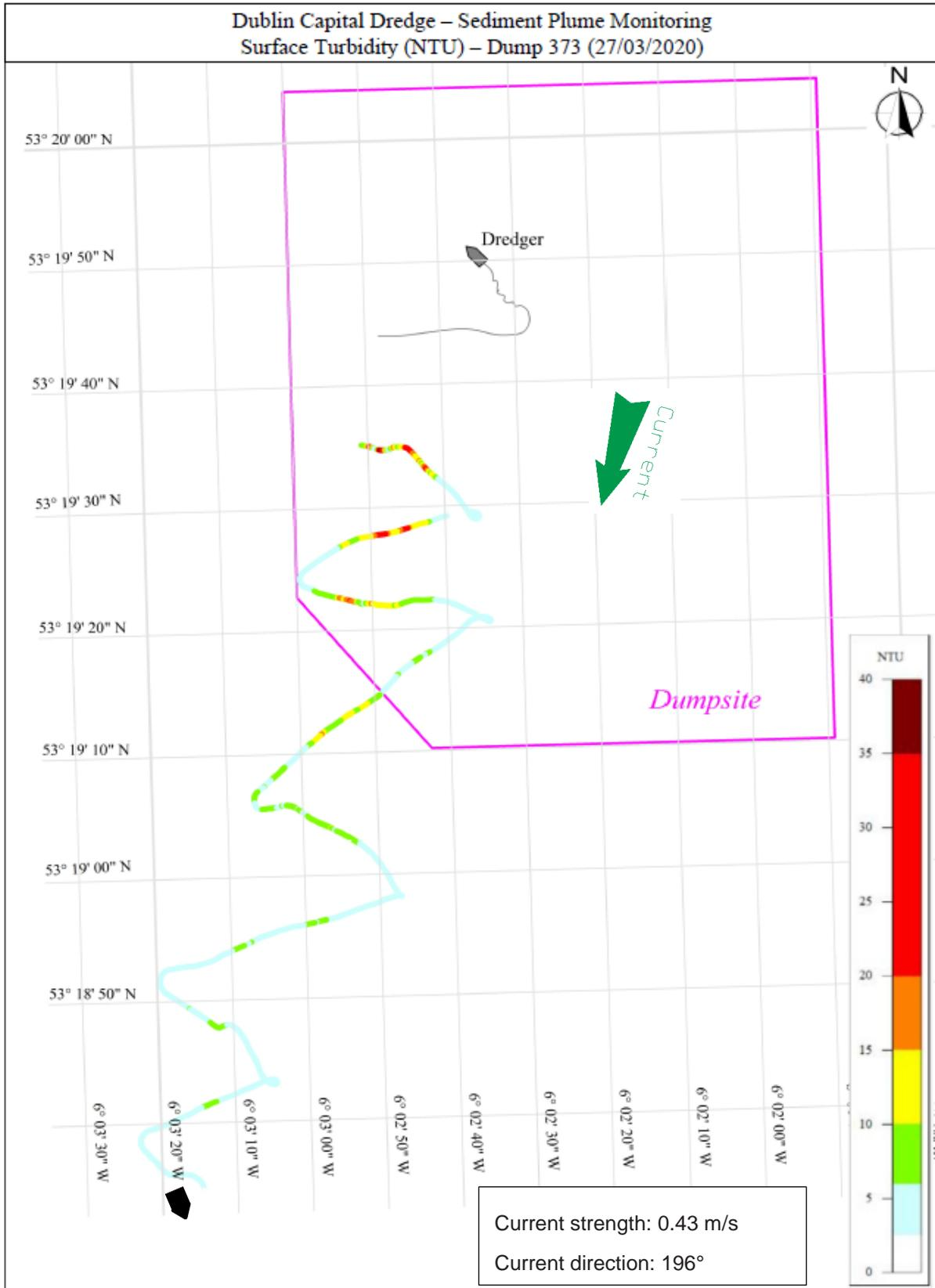
**Figure 8.26: Dump 373 Survey track with surface turbidity [NTU]**
