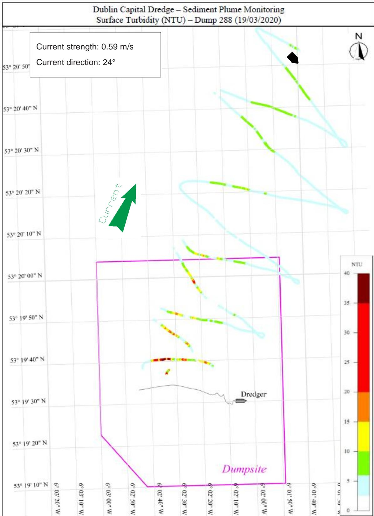
**Figure 8.23: Dump 288 Survey track with surface turbidity [NTU]**
