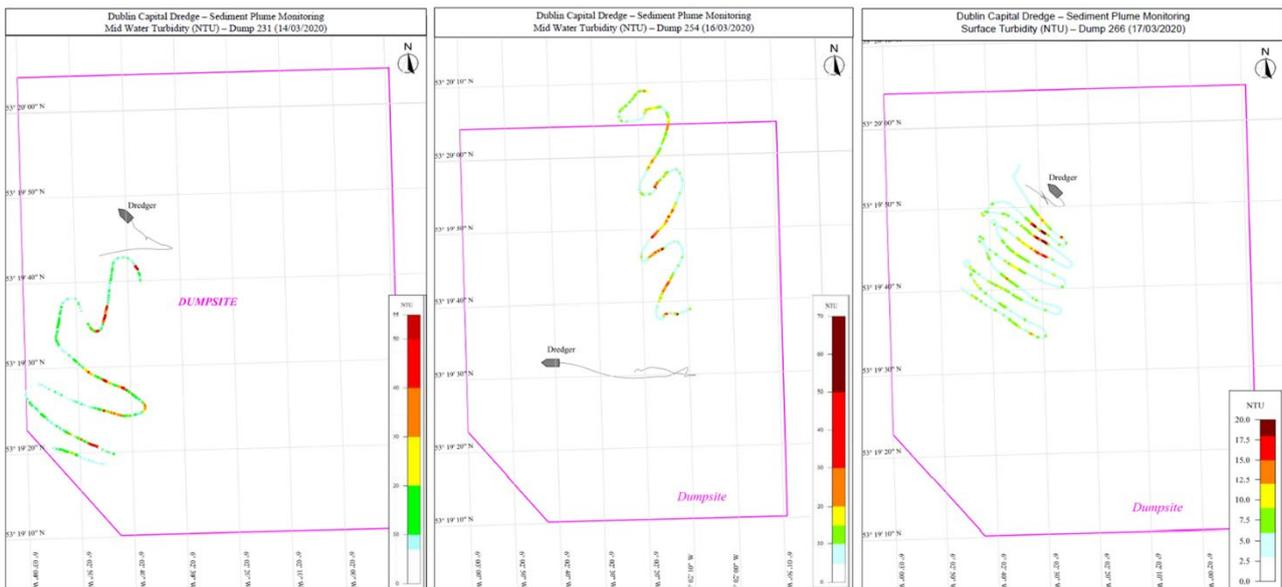
**Figure 4-2 TSHD track during the disposal of sediment across three individual dumping activities (trips) with the corresponding measured suspended sediment concentration**
