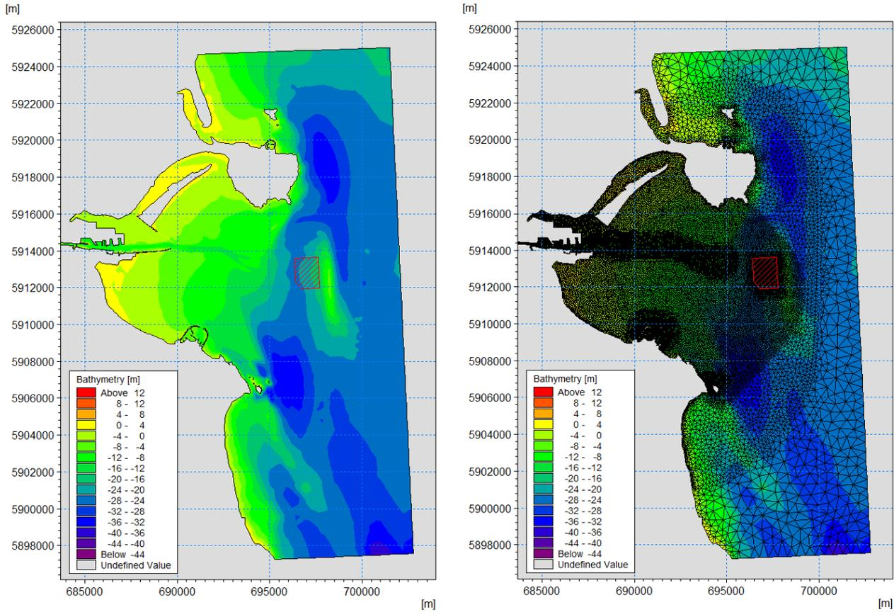
Figure 4-4 Extent and bathymetry (left) and mesh structure (right) of the Dublin Bay model. Location of the licenced dump site shown by red hatch area.
