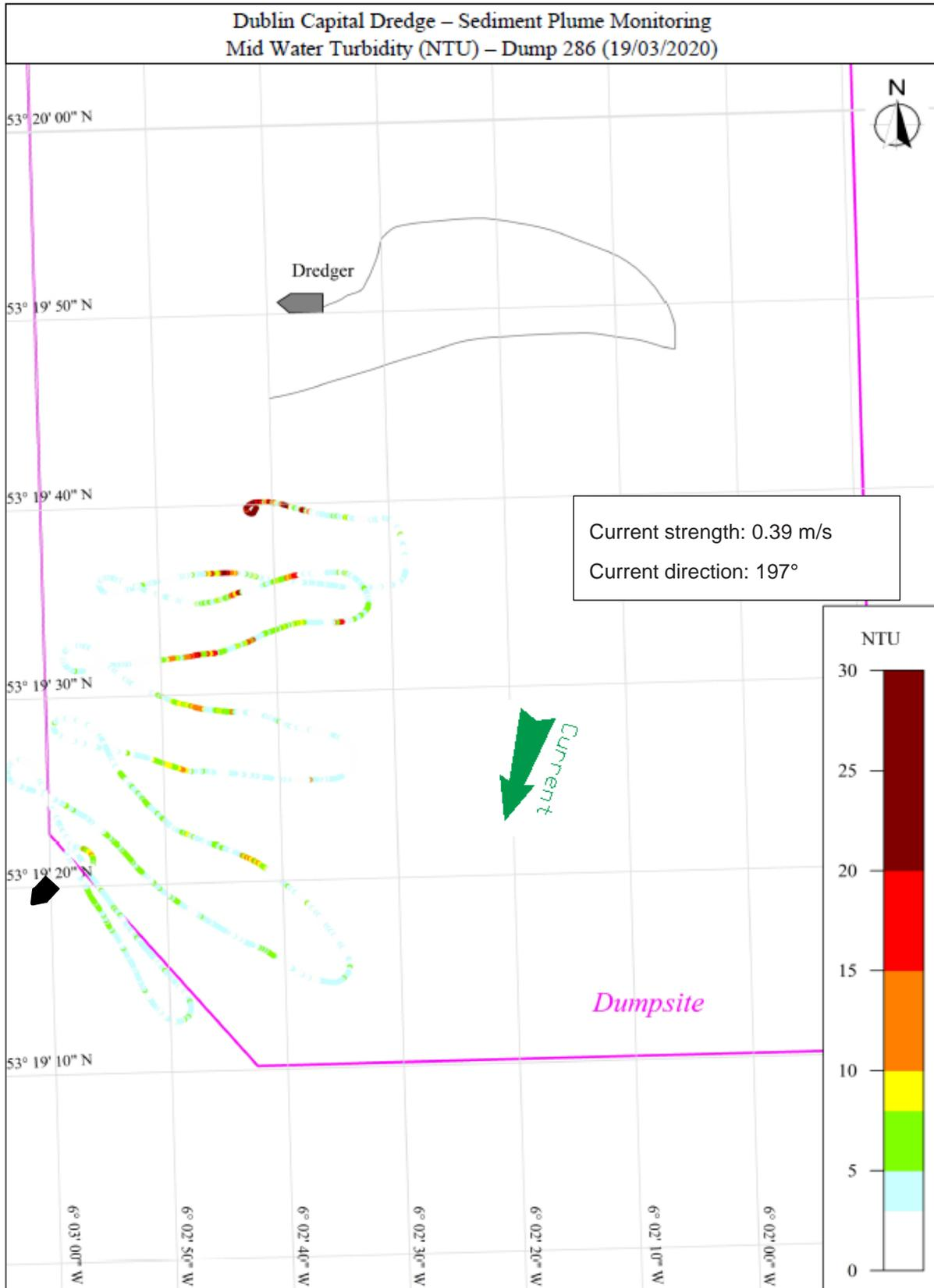
Figure 8.20: Dump 286 Survey track with mid water turbidity [NTU]
