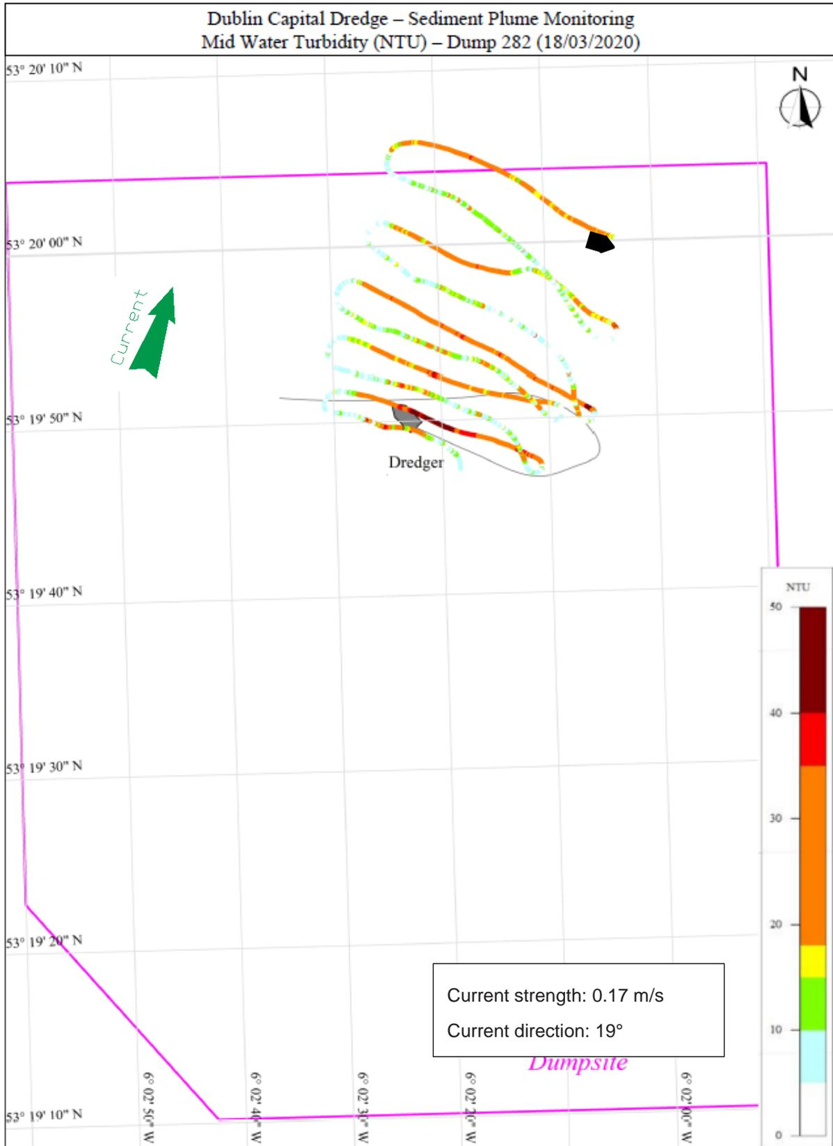
Figure 8.13: Dump 282 Survey track with mid water turbidity [NTU]
