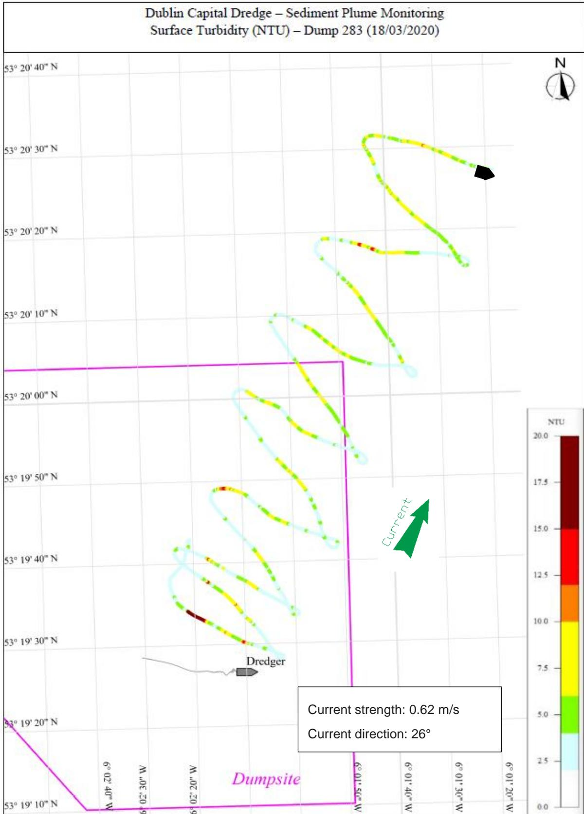
**Figure 8.14: Dump 283 Survey track with surface turbidity [NTU]**
