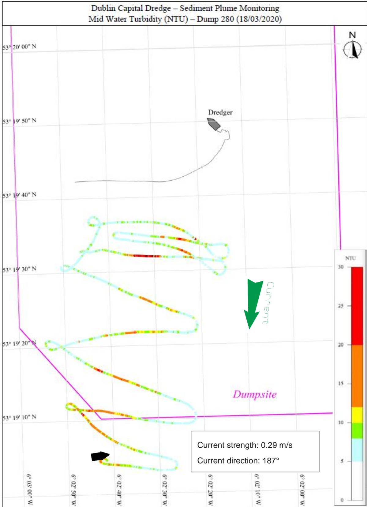
Figure 8.10: Dump 280 Survey track with mid water turbidity [NTU]
