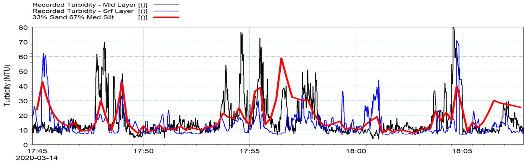
Figure 5.4: Comparison of recorded and simulated turbidity levels during dump event 231 – Mixture 3 (33% fine sand; 67% medium silt)
