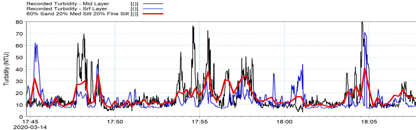
Figure 5.3: Comparison of recorded and simulated turbidity levels during dump event 231 – Mixture 2 (60% fine sand; 20% medium silt; 20% fine silt)
